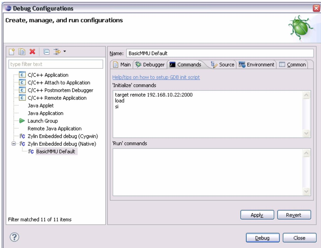
The **target remote** command tells to gdb to connect to PEEDI using the provided IP address. The **load** command loads the code to be debugged to the target (in this case it loads it to the RAM). The **si** command tells the gdb to make a single step just to refresh the eclipse debug view. After finished click **Debug**, this will start a debug session and eclipse will ask you to witch to debug perspective, click **Remember my decision** and then Yes:
