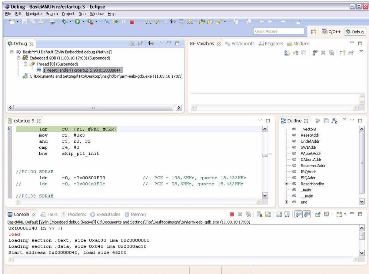
Now you can continue debugging normally, i.e. do some single steps, put breaks or hit the resume button to start the executions. You can insert a break clicking on the beginning of the desired line in the source file, for example I will click on the C/C++ perspective just to see the source files, so I can open `init.c`, then I will switch back to the debug perspective and put a break on the first line of `AT91F_LowLevelInit()` function:
