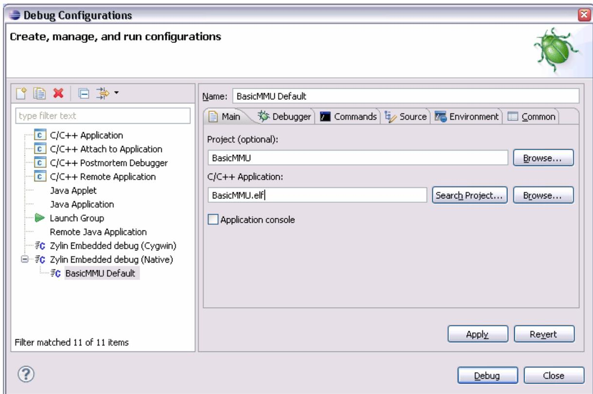
Next open the debugger tab and make sure the right gdb is selected as **GDB debugger**, for ARM targets it should be `arm-xxx-gdb`, for example `arm-elf-gdb`, `arm-none-gnueabi-gdb` or just the `gdb` that comes with your GCC toolchain. If the selected debugger is not found because its path is not set correctly, you can use the **Browse** button to exactly point to it and thus exclude any path problems. Next open the **Commands** tab and fill it like this considering your PEEDI IP:
