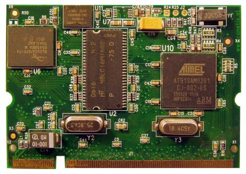
The PM9261 from Ronetix consists of an AT91SAM9261 together with several peripherals:
